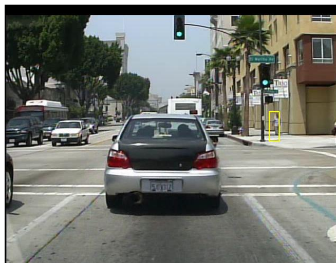
Fig. 8. Pedestrian detection results using Faster RCNN approach.
