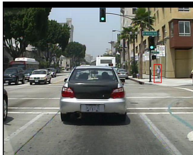
Fig. 7. Pedestrian detection results using SSD approach.
