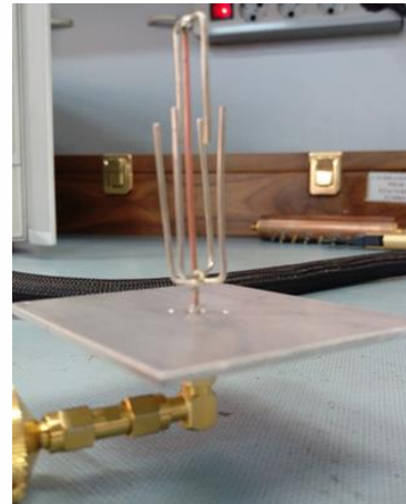
Figure 2. Fabricated multi-band monopole antenna.
