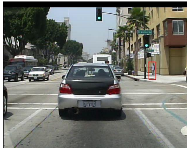
Fig. 7. Pedestrian detection results using SSD approach.
