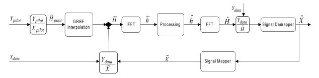
Figure 5. Channel Estimation and Detection structure block diagram for OFDM system.
