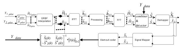
Figure 6. Channel Estimation and Detection structure block diagram.
