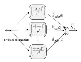
Figure 7. GRBFN structure for Channel Estimation.
