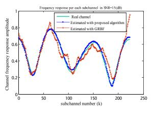
Figure 15. channel frequency response amplitude.
