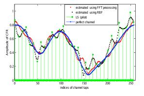
Figure 14. channel frequency response amplitude.
