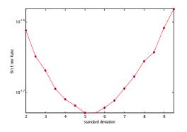
Figure 9. BER of our proposed algorithm in terms of standard deviation.
