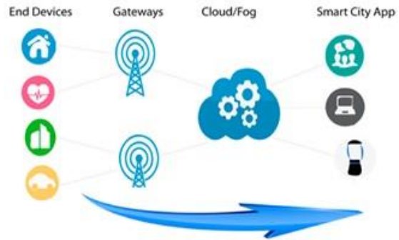
Fig. 2. LoRa-based IoT ecosystem
