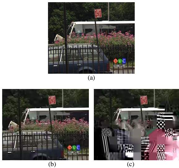
Fig. 12. Screenshot comparison for “Bus” video sequence; (a) original sequence, (b) noisy video sequence transmitted and reconstructed with adaptive modulation case, (c) noisy video sequence transmitted and reconstructed with constant modulation depth.
