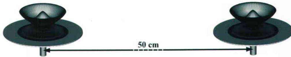
Fig. 18. A pair of second optimized antennas placed 50 cm away from each other in free space which are operating as transmitter and receiver.
