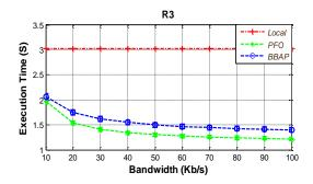
Fig 3. Bandwidth Impact on execution time using R3
