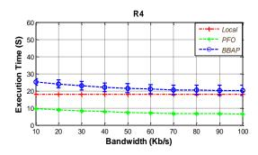
Fig 5. Bandwidth Impact on execution time using R4
